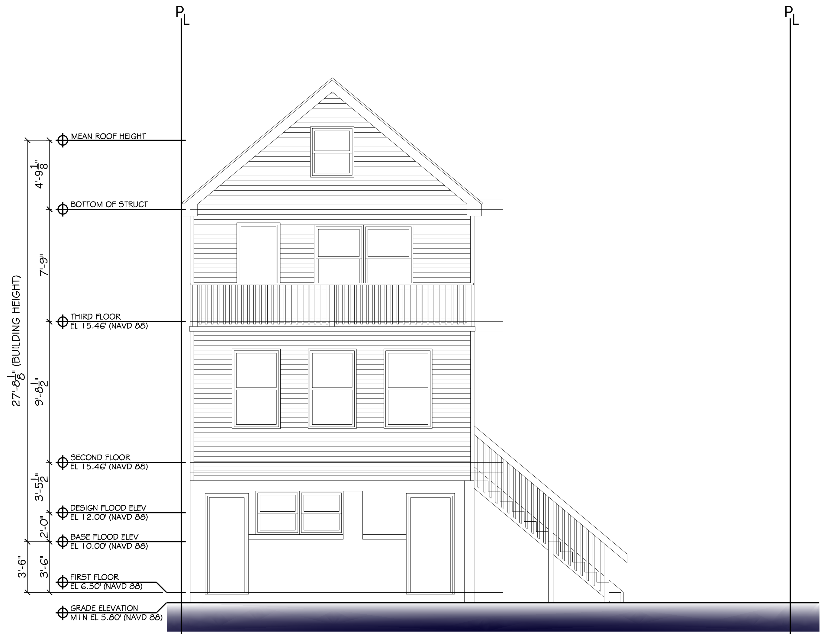
EXISTING FRONT ELEVATION (TEXAS ELEVATION)
