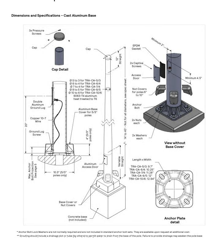
NOTE: Factory supplied template must be used when setting anchor bolts. Gardco will not honor any claim for incorrect anchorage placement from failure to use factory supplied
