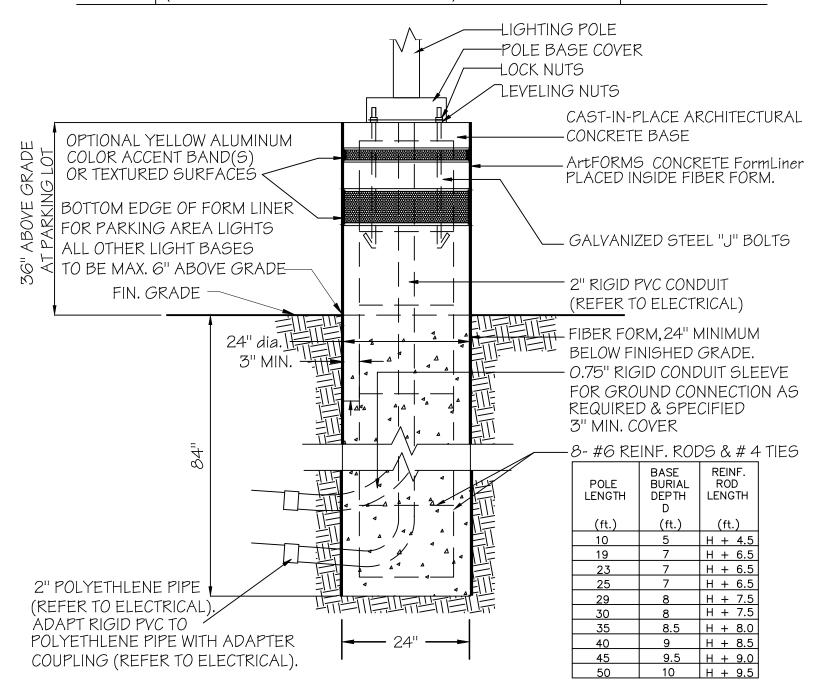
NOTE: DEPTH OF FOOTING TO BE VERIFIED BY THE STRUCTURAL ENGINEER UPON REVIEW OF SOIL BORINGS. LIGHT POLE BASE
