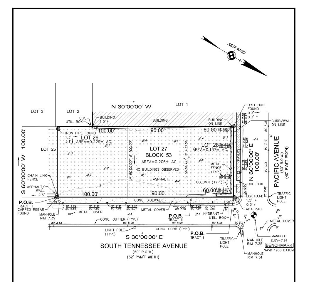
NOTE: VERTICAL DATUM IS NAVD88 ESTABLISHED THROUGH LEICA RTK GPS NETWORK.
