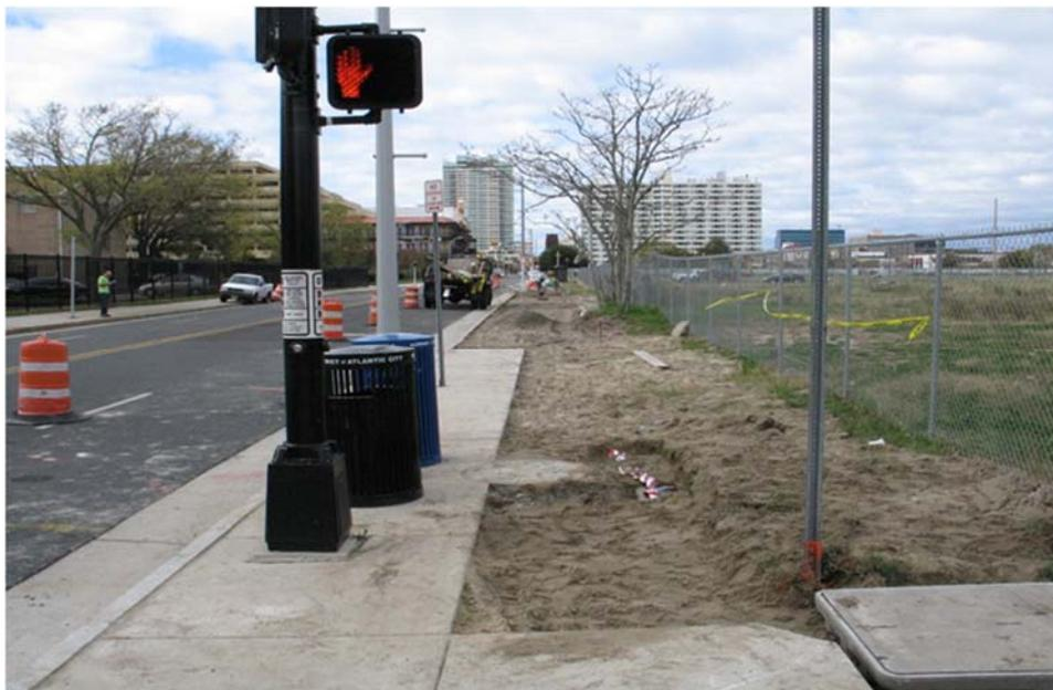
*Looking West along Pacific Avenue from the Connecticut Avenue intersection. Block 132 on the Right. As per current ADA, the cross-slopes of existing and proposed sidewalks will need to be addressed on the plans, adhering to the maximum cross-slope of 2.0-percent.*
